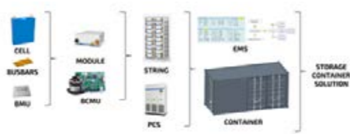
Figure 34: Internal components of a battery
